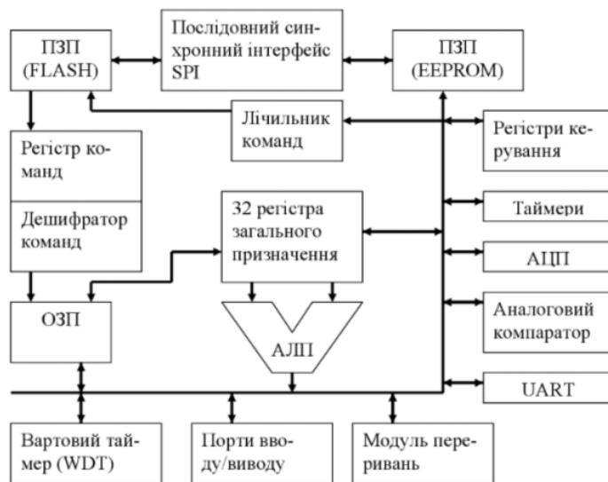
Fig. 2. Typical kernel architecture of AVR microcontrollers [6].
