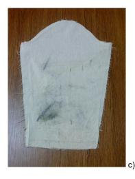
**Figure 2** Details of prototypes of the children's clothes with the graphite contamination in the places where child's body in the prototyped clothes contacted with the impact surface: a) back half of the trousers; b) front half of the trousers; c) sleeve
