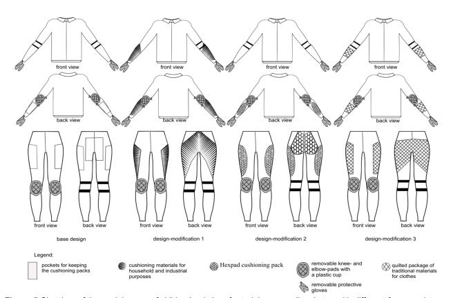
Figure 5 Sketches of the model range of children's clothes for trainings on roller-skates with different forms and types of protective elements
